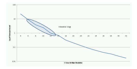
Figure 7.8: 3-Torus complexity vs. log(frames-per-second) Frame rates determined from internal software profiling.
