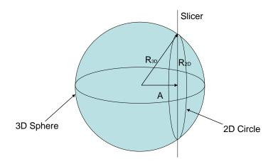
Figure 7.5: Plucking a 1-sphere (2D circle) from a 2-sphere (3D sphere) A plane intersects a sphere of radius  $radius_{3D}$  ( $R_{3D}$ ) at position A along the Z axis scribing a circle of radius  $radius_{2D}$  ( $R_{2D}$ ).
