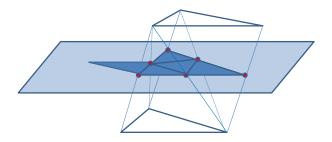
Figure 6.6: Plucking a Triangular Mesh from a Tetrahedral Mesh. simplicial 2-complex which will be rendered. A pseudo-code description of this process is given in Figure 6.14.
