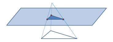
Figure 6.5: Constructing a Triangle from Intersected Tetrahedral Edges.
