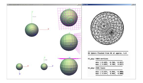
Figure 7.6: Plucking a 2-sphere (sphere) from a 3-sphere (hypersphere) A plane intersects a 3-sphere of radius  $radius_{4D}$  at position *B* along the *W* axis scribing a sphere of radius  $radius_{3D}$ . The radius of the 4D sphere at intersection is selected via the icon to be ~ 4.0 world-units. The 3D .ply Viewer confirmed a radius of 3.971 world-units.
